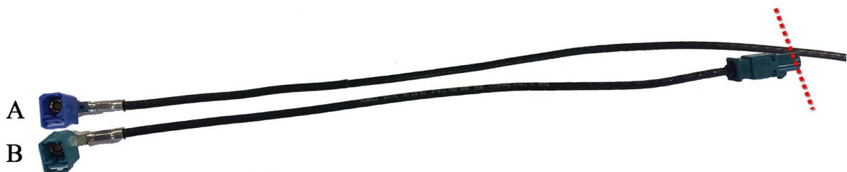
Figure 2. Measure you're the cut point on the vehicle's antenna coaxial wiring (A) based off the length of the replacement coaxial "Adapter Antenna Cable" (B). The removed length of cable from A should be equal to the length of cable B.
