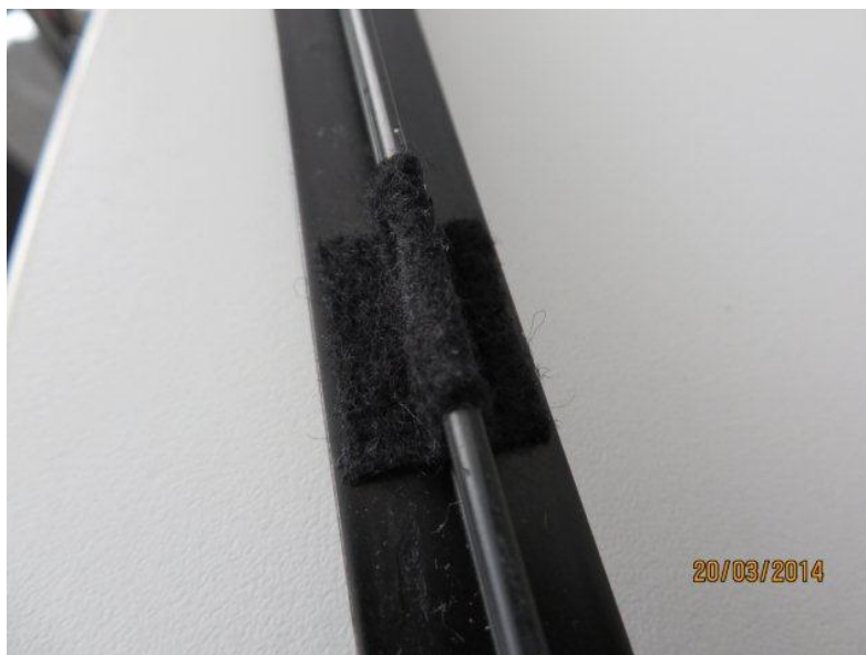
Figure 3. Fleece adhesive tape section applied.
