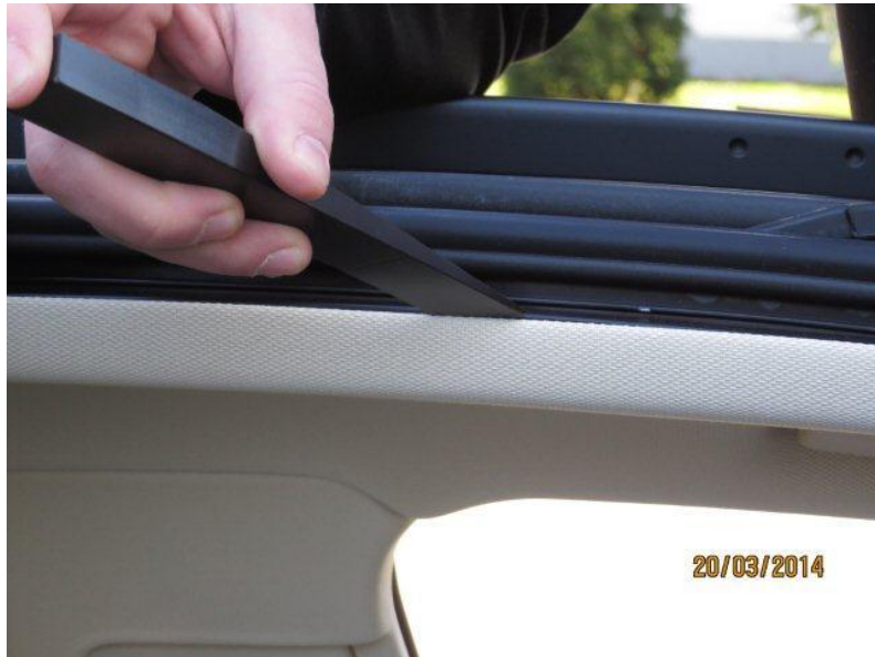
Figure 1. Unclipping the sunroof cover trim frame.
