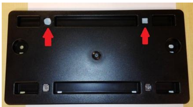
Figure 1. Damaged screw inserts.
