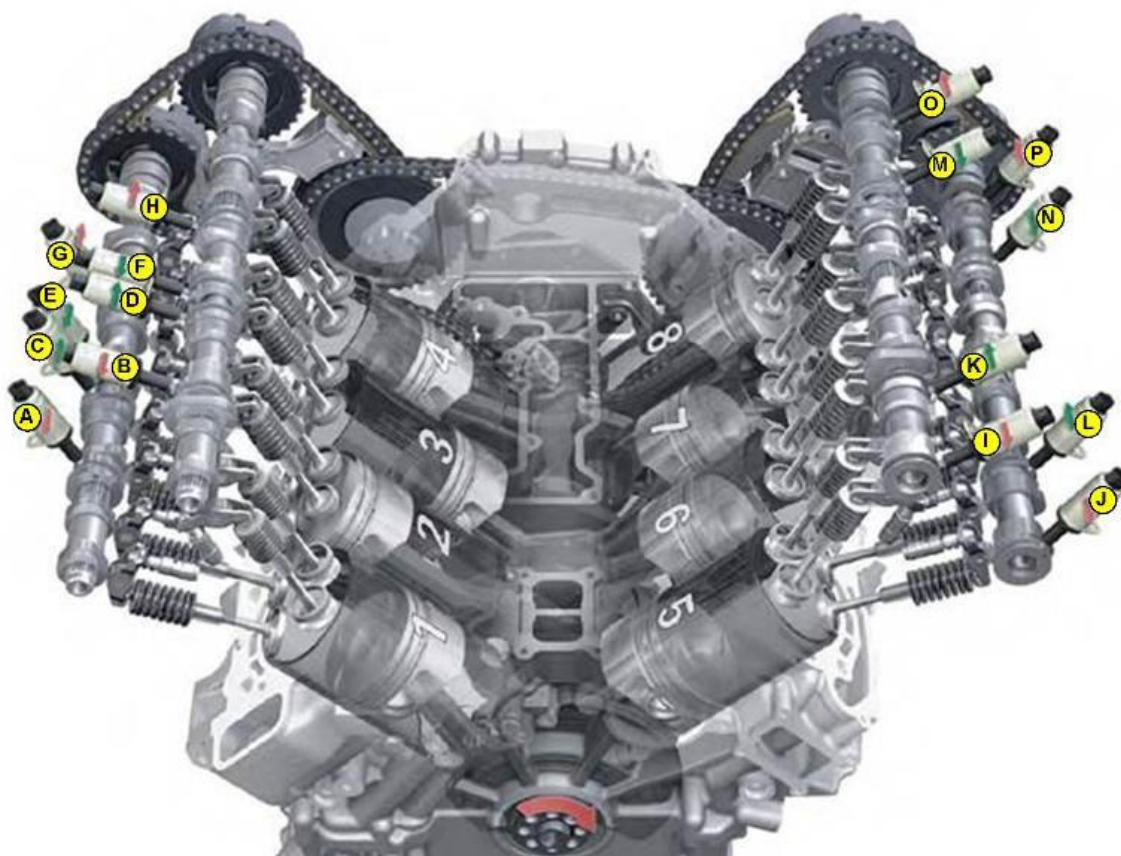
Figure 1. Use this image to identify the installation position of the affected actuator.
