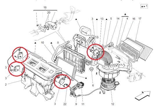
To resolve this issue, a new software version for the HVAC ECU is now available. The new software will improve the motor management for the air flow control actuators to help prevent them from getting stuck.
