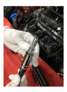
8 Tighten all 4 spark plugs with a torque wrench to specifications.
