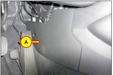
• Then slide the LH console side cover (A) towards the rear of the vehicle to remove the cover.
