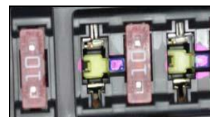
Loose Fit Between Fuse terminals
