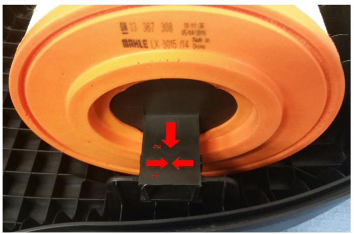
**Important:** When removing the air cleaner element, care should be taken not to damage the bracket mount. Follow the instructions on the bracket for air filter removal.
