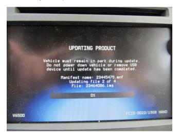
4. DO NOT remove the USB drive until the update has been completed. Once the update has been completed, the display will go black for a minute, reset itself and then display the start-up screen. At this point, remove the USB flash drive, turn the ignition off, open the driver's do and close the driver's door to allow the radio to go to sleep.
