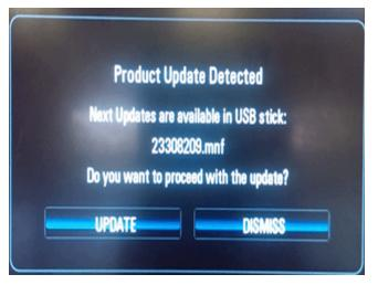
**Note:** If "UPDATE" is not selected within 10 seconds, the screen will disappear and the USB drive will have to be removed and inserted again to start the update process over again.
