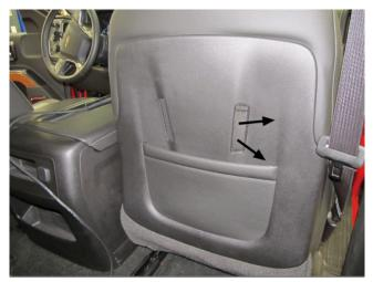
The cause of this condition may be that during cooled seat operation, a direct flow of warm air exhausts from the upper seat back ventilation heating/cooling blower thermal exchange blower unit.
