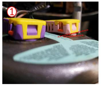
In the example above, it was found that the connector was not locked in completely (1), causing the wiring to move or lose connection while vehicle was moving.
