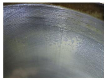
Some technicians may be replacing entire engine assemblies due to marks found at the top of the cylinder bore.
