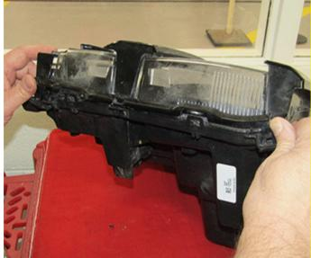
Important: To avoid damaging the bezel, gently push upward in a uniform manner, without twisting the bezel. This should release the attachment tape from the loose side across to the opposite side and the bezel can be
