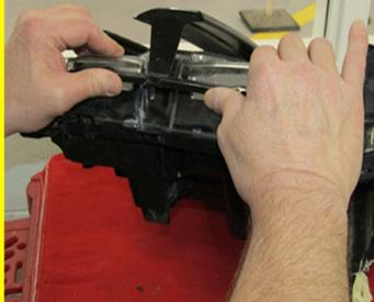
3. Grabbing the top and bottom corners of the loose side of the headlamp bezel, carefully push the bezel upward to release the remaining tape holding the bezel to the lamp.
