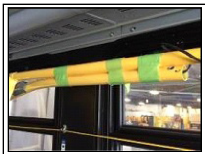
Figure 12 - Typical View of Securing the Stanchion
