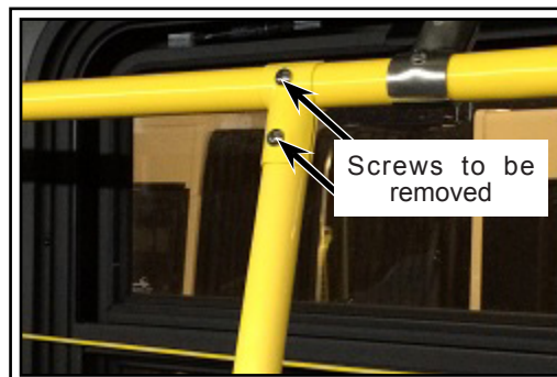
Figure 9 - Removal of Screws on the Stanchion
