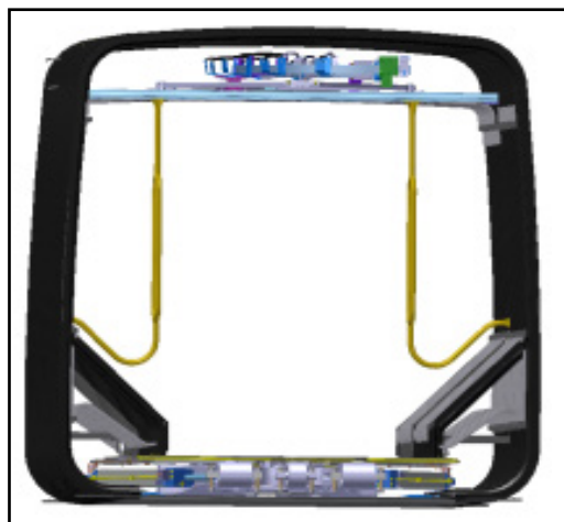
Figure 2 - Typical View of Articulation System Inside the Vehicle
