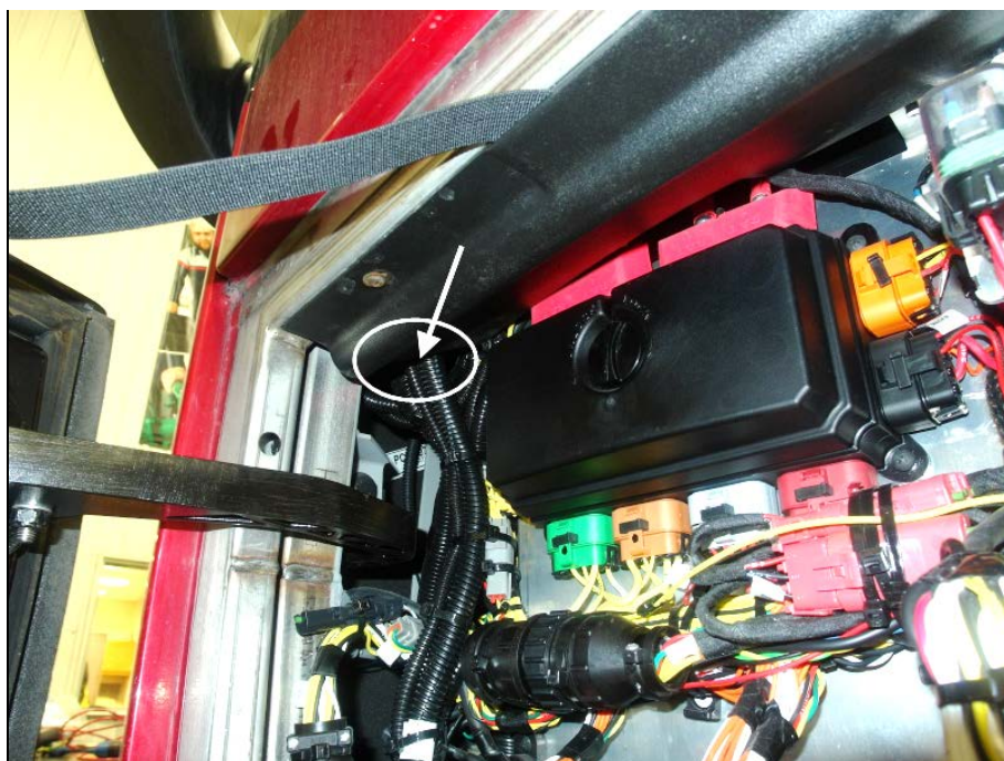
AVOID CONTACT HERE ON H3 VEHICLES
