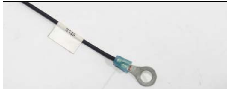
ROUND TERMINAL ON GROUND WIRE
