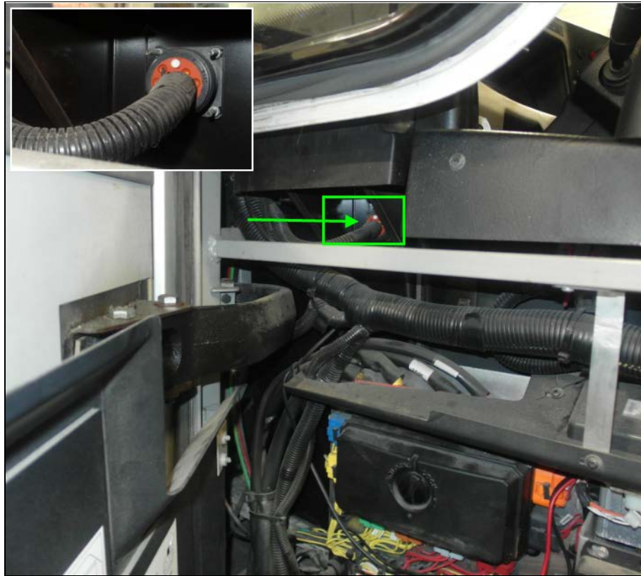
DIAGNOSTIC CONNECTOR POSITION (X3 VEHICLES)
