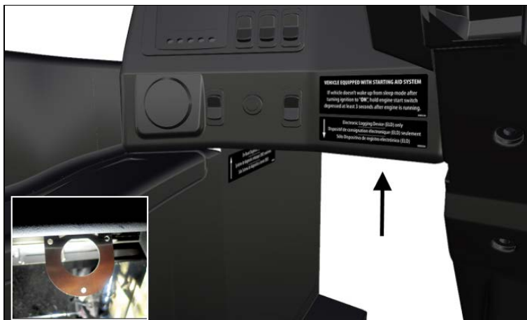
BRACKET POSITION UNDER DASH
