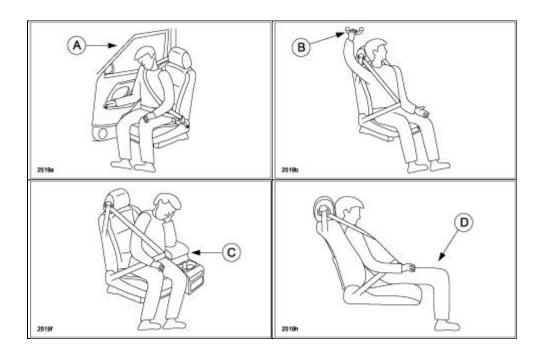
In the examples above, the PAD indicator illuminates when the value detected by the sensors becomes less than the weight threshold. Also, a front seat passenger who weighs near the airbag's cutoff threshold can cause the PAD indicator illumination to turn on and off intermittently.
