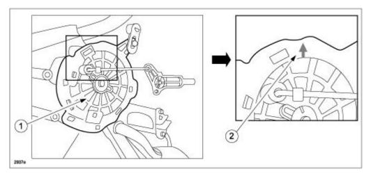
b. Disconnect the rod from the air flow mode main link.
