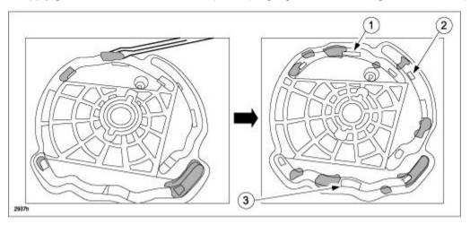
f. Install the air flow mode main link (with marked arrow (1) pointing upward) and engage the link for each mode door into the respective air flow mode main link channel.
