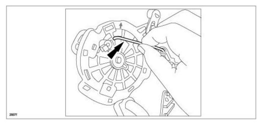
c. Remove the screw (1), then remove the air flow mode main link (2).
