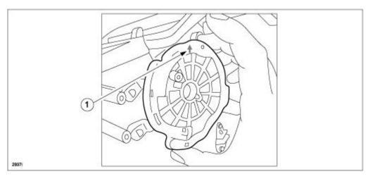
g. Install the collar (1) and tighten the screw.
