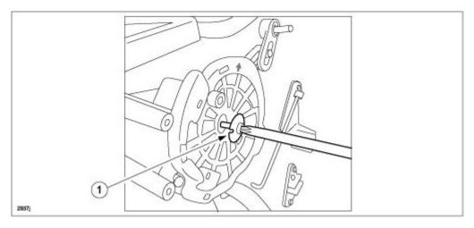
h. Rotate the air flow mode main link (1) several times back and forth between the "VENT" and "DEF" positions to verify the mode can be switched properly.
