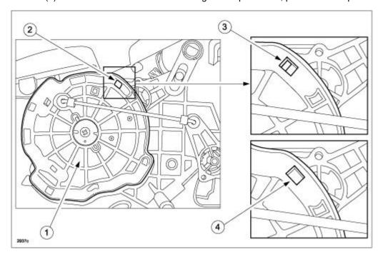
5. Remove the E-ring (1) at the tip of the mode selector wire and reinstall it to a maximum of 2 mm away (2) from the original position (3), as shown below.
