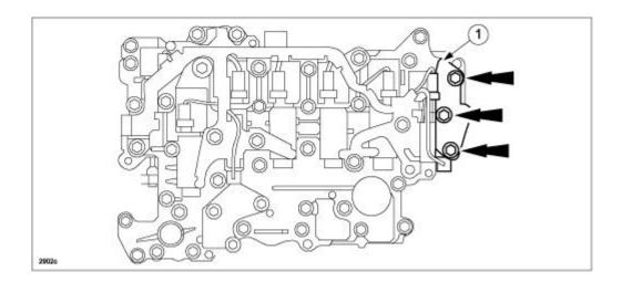
c. Detach the tab shown and remove oil pressure switch A from the control valve body using an appropriate tool (such as a fastener remover)
