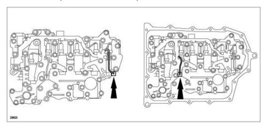
9. Install the oil strainer with new oil strainer O-rings according to the instructions on MGSS online (CONTROL VALVE BODY REMOVAL/INSTALLATION [FW6AEL, FWAX-EL]).
