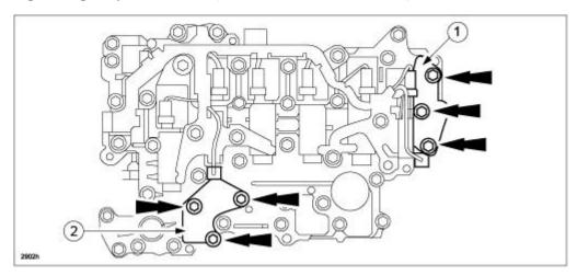
8. Connect the oil pressure switch A and oil pressure switch B connectors.
