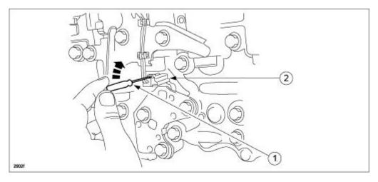
b. Remove oil pressure switch B (1).
