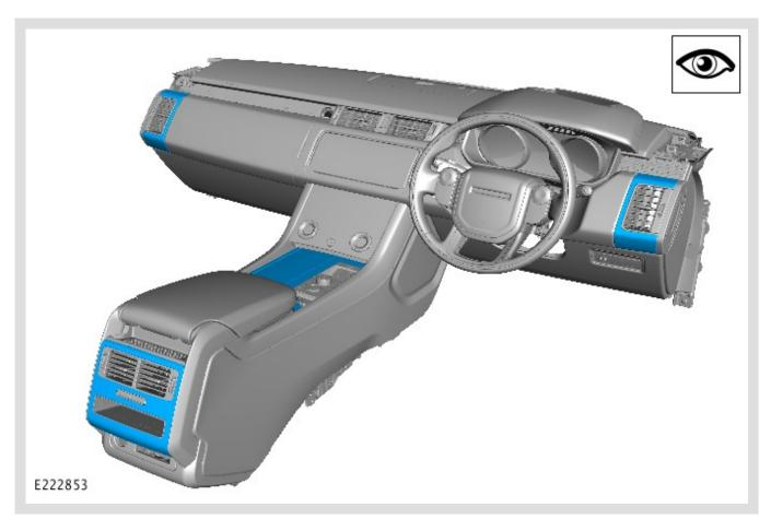
Inspect the floor console and instrument panel veneer inserts for scratches.
