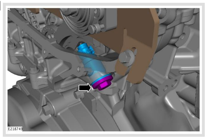
Install the upper timing chain tensioner.
