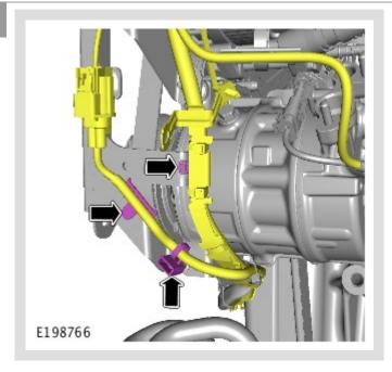
Position the wiring in place.
