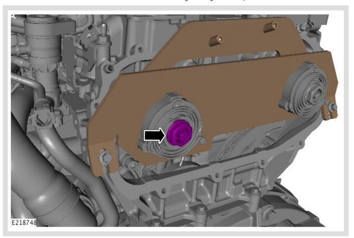
Loosen but do not fully remove the VCT actuator fastener.
