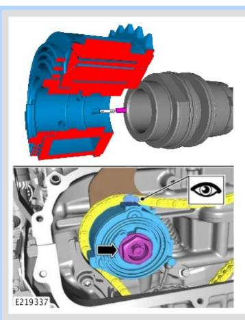
Install the new intake camshaft VCT actuator and fastener.
