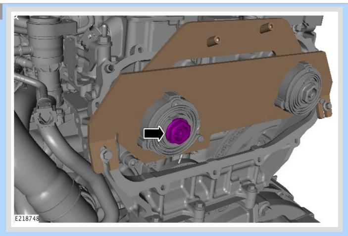
Tighten the intake camshaft VCT actuator fastener.
