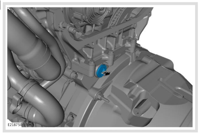
Use a suitable tool to remove the lower timing cover blanking plug.
