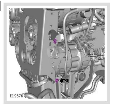
Install the charge air cooler bracket fasteners.
