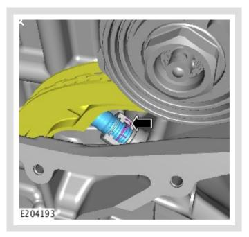
Release the upper timing chain tensioner piston.
