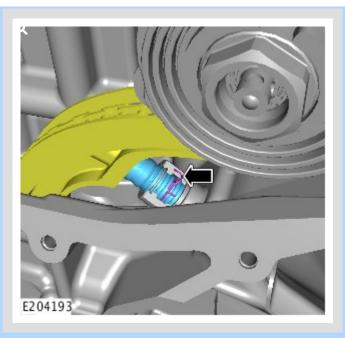
Release the upper timing chain tensioner piston.
