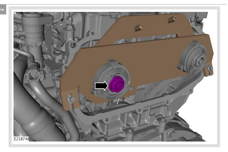
Tighten the intake camshaft VCT actuator fastener.
