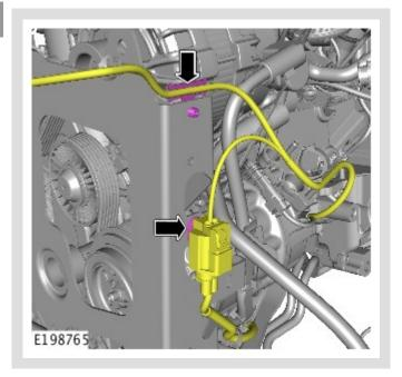
Release the wiring.
