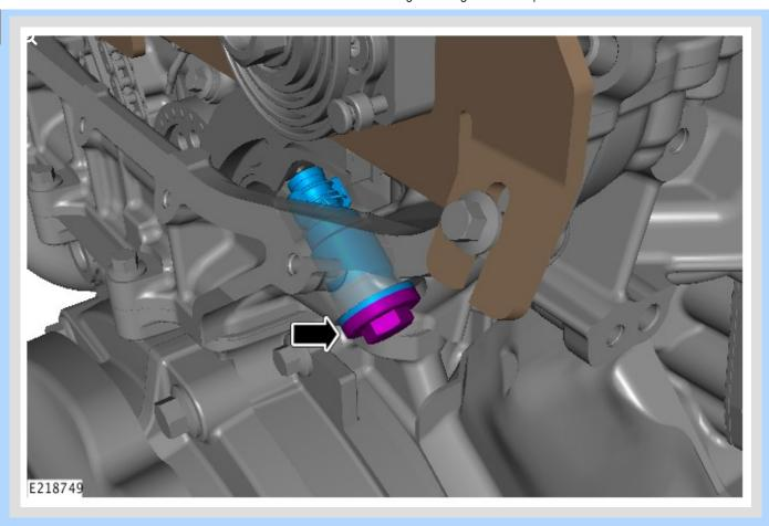
Install the upper timing chain tensioner.
