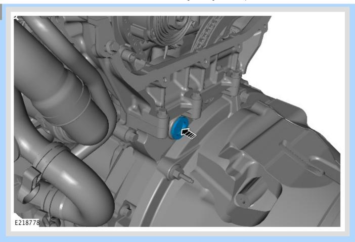
Install a new lower timing cover blanking plug.
