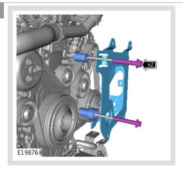
Remove the charge air cooler bracket.
