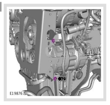
Remove the charge air cooler bracket fasteners.
