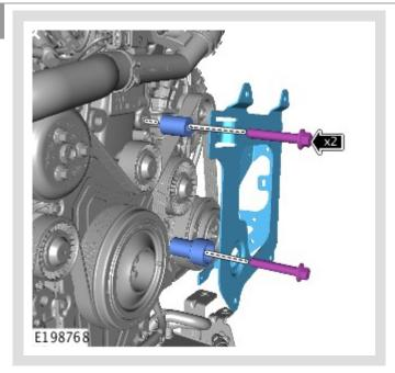
Install the charge air cooler bracket.
