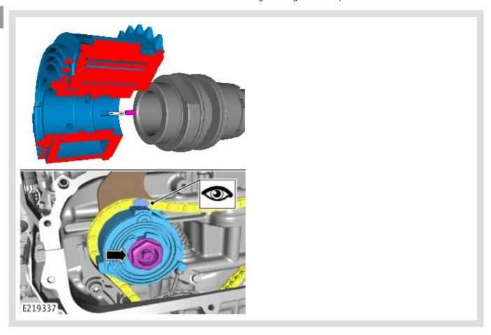
Install the new intake camshaft VCT actuator and fastener.
