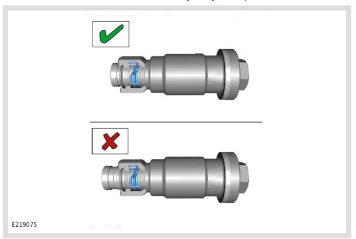
Make sure the upper timing chain tensioner is compressed as shown  $[\checkmark]$  before installing.
