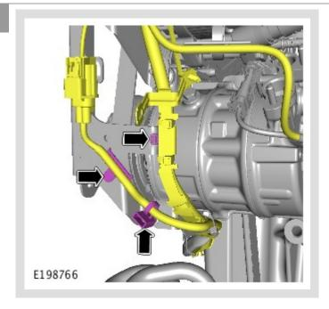
Release the wiring.
