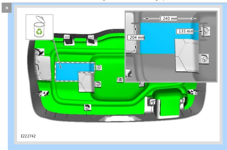
Use a suitable knife to carefully remove a section of the Noise, Vibration and Harshness (NVH) material from the tailgate trim panel as shown.
