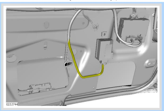
Position the wiper relay suppression module wiring harness to the side.
