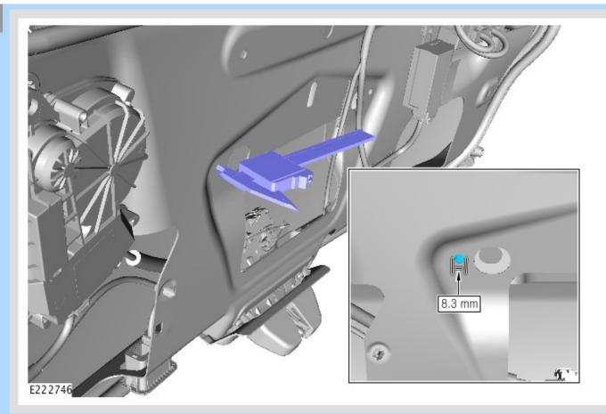
Use a suitable tool to measure the diameter of the hole for the tailgate trim panel retaining clip in the tailgate.
