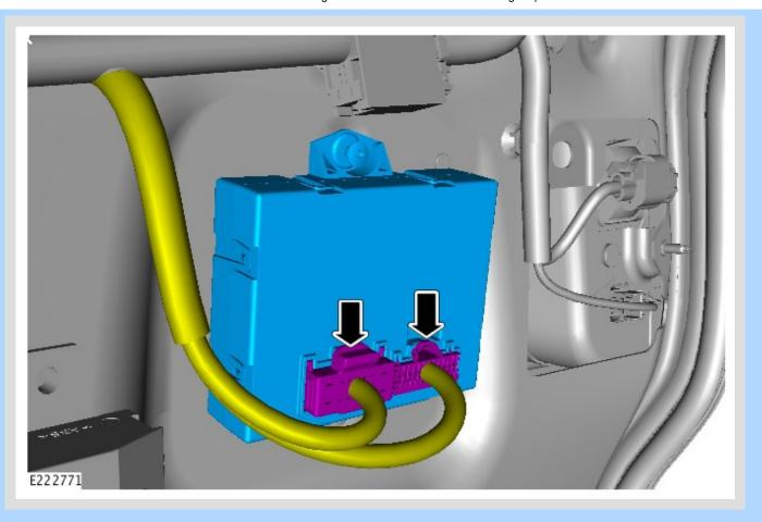
Connect the electrical wiring harness to the power tailgate module.
