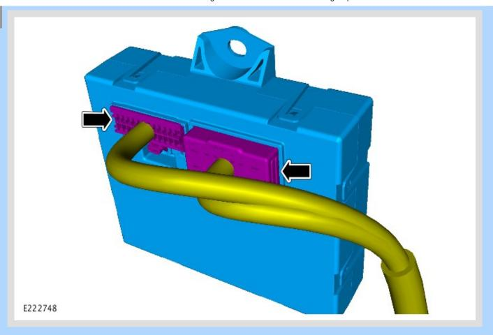
Disconnect the power tailgate module and position the electrical wiring harness to one side.
