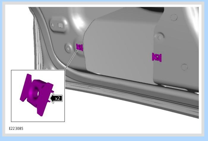
Install the 2 new retaining clips.
