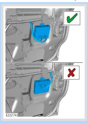
The power tailgate module must be installed with the electrical connectors towards the bottom of the tailgate.
