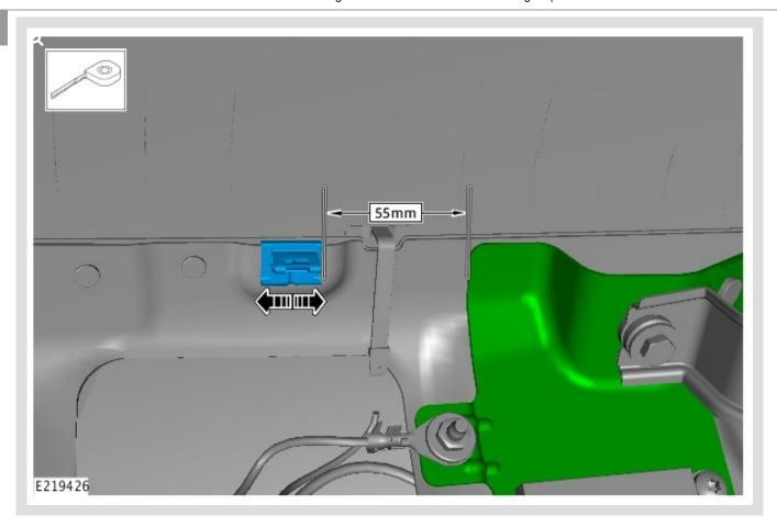
Adjust the position of the new tailgate clip as shown.
