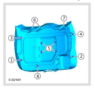
Install the 9 new tailgate trim panel clips into the tailgate in the order shown.
