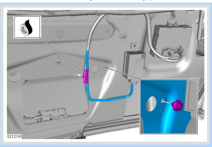
Secure the wiper relay suppression module wiring harness to the tailgate wiring harness with suitable electrical tape.
