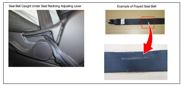
The shape of the seat reclining adjusting lever has been modified to prevent fraying of the seat belt should it get caught under the lever.
