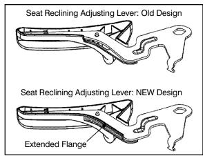
2. Confirm the replacement seat reclining adjusting lever is the new countermeasure part.
