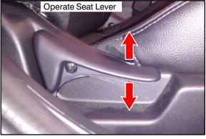
6. Operate the seat reclining adjusting lever and confirm smooth operation.
