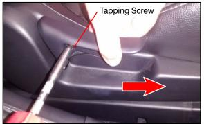
3. Remove the tapping screw, then pull out the seat lever to the front of the vehicle and remove it.
