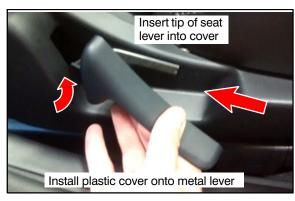
4. Install the plastic cover of the new seat reclining adjusting lever onto the metal lever as shown.
