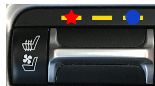
B+ Power Fault
