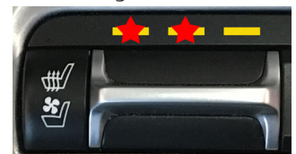
Short Circuit in Blower Motor Signal Wire
