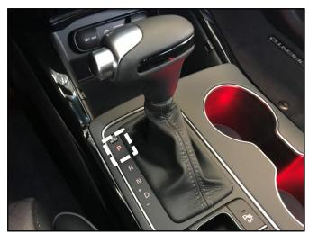
6. With the vehicle in "Park", push on the accelerator pedal fully, wide-open throttle (WOT) at approximately 4,500 – 5,500 RPM, for two (2) seconds and then release the accelerator pedal and let the engine idle for one (1) second. NOTE: during this step, listen for abnormal engine noises.
