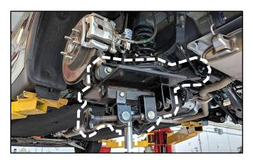
3. Remove the retaining lower shock bolt (A) and the stabilizer link bolt (B).
