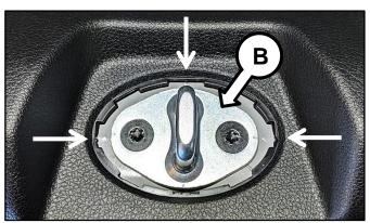
3. Remove the two (2) transverse trim clips (C) using a small pick tool and pull the cover off from inside the rear trunk.
