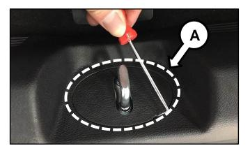
Inspect the alignment marks on both the body and the striker (B). The markers must be aligned to match. If so, reinstall the striker cover to complete the inspection. Road test vehicle on rough road to confirm no rattle noise is present.
