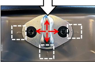
7. Once adjusted, torque striker mounting bolts to specifications and ensure tailgate door latches to striker properly.
