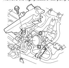
5. Remove the quick-connect fitting cover.
