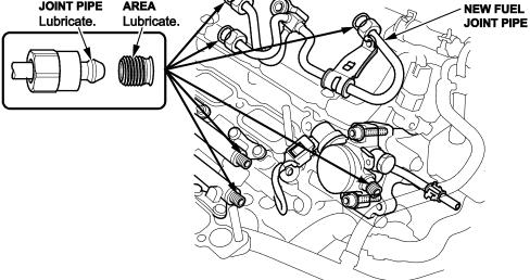
20. Tighten the fuel joint pipe nuts by hand until the end of the joint pipe is seated on the fuel rails and high pressure fuel pump.
