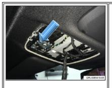
Remove the FZD to inspect the sunroof drive motor following repair instructions REP 61 31 043 Removing and installing the FZD.
