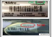
2. Inspect the identification label number on the sunroof drive motor. The identification number is located in the top right corner of the label as shown.
