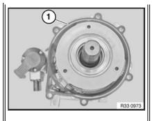
Both halves of the QMVH (1) will need to be resealed during the repair (do not repair only the side that is leaking).
