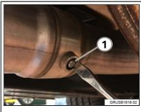
3. If the flap is operating as designed (closes fully and fixing bow is installed), apply pressure to the bushing of the flap. If the rattle goes away, replace the rear muffler with exhaust flap. **NOTE:** If the flap is rattling due to the software error, the rattle will also go away when applying pressure to the bushing. Check for the software issue first before diagnosing the bushing and replacing the rear muffler.
