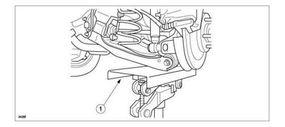
12. Tighten the rear lower arm outer bolt to the specified torque.
