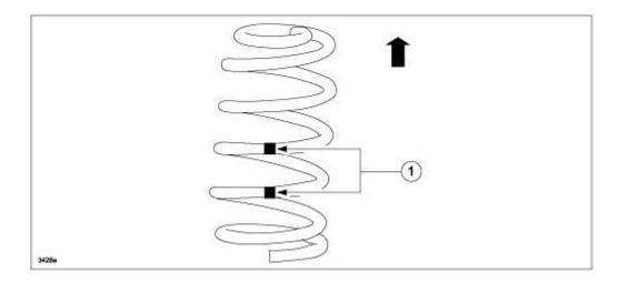
9. Align the upper end of the rear coil spring with the upper spring seat rubber.
