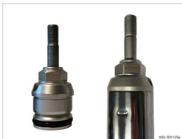
Fig. 2: Version 2 - Fixed fork tube with pressed in seal plugs with oval crimps.
