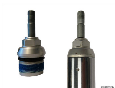
Fig. 1: Version 1 - Fixed fork tube with threaded plug with circular indentations
