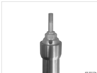
Fig. 3: Version 3 - Fixed fork tube with pressed on fixed fork tube bushing
