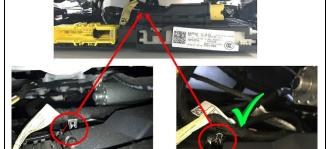
8. Secure the loose clip attached to cables, as shown.
