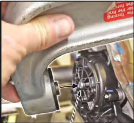
Place the tool on the pinion shaft of the VTA unit.
