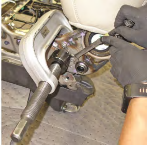
Tighten the tool until the VTA unit shaft protrudes.
