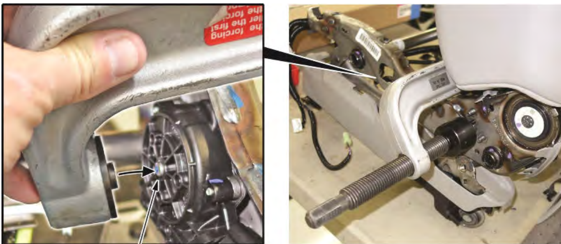
Place the tool on the pinion shaft of the VTA unit.
