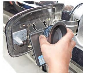
3. Press the bottom of the fuel lid cover to the fuel door until both locking tabs click. This indicates the fuel lid cover is securely and correctly installed.
