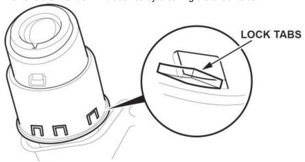
2. Pry up the lock tab and remove the mis-fuel inhibit device.
