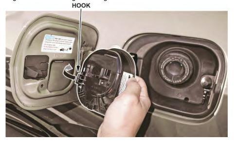
3. Press the left of the fuel lid cover to the fuel door until both locking tabs click. This indicates the fuel lid cover is securely and correctly installed.
