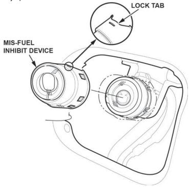
3. Install the new mis-fuel inhibit device.
