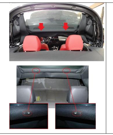
Verify that holes have been worn through the headliner, above the rear window in the area shown to the left.
