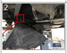
2. Inspect the plastic nuts securing the underbody panel bracket in the area shown in photos 2&3. Photo 3 shows an example of a bracket that is missing 1 of the plastic nuts.
