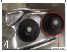
3. If either bracket nut is found to be loose or missing, re torque or install the plastic nut to 2.6 Nm. There should be 2 plastic nuts installed for each bracket as shown in example photo 4.
