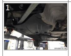
4. Reinstall the underbody panel, torqueing the screws to 3 Nm.
