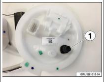
Install the locking cap (PN 16 11 7 462 535) on to the open auxiliary port (1).
