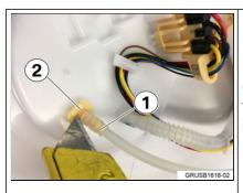
Carefully cut the parked car heating line (1) from the underside of the fuel pump mounting flange (2) (this section of fuel line is no longer needed).
