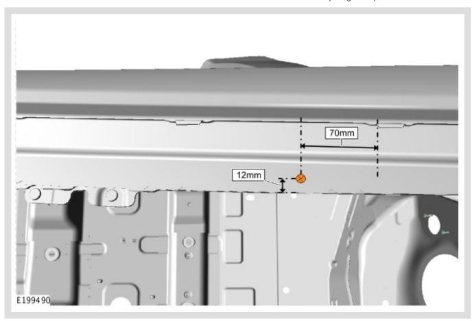
Install a Self Piercing Rivet (SPR) between the roof/cantrail inner panel/cantrail outer panel in the position shown.
