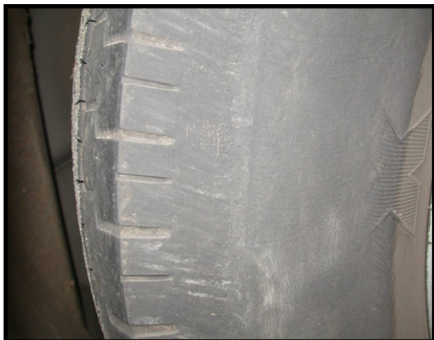
WORN SIDEWALL LETTERING DUE TO SCRUB, ROTATION REQUIRED
