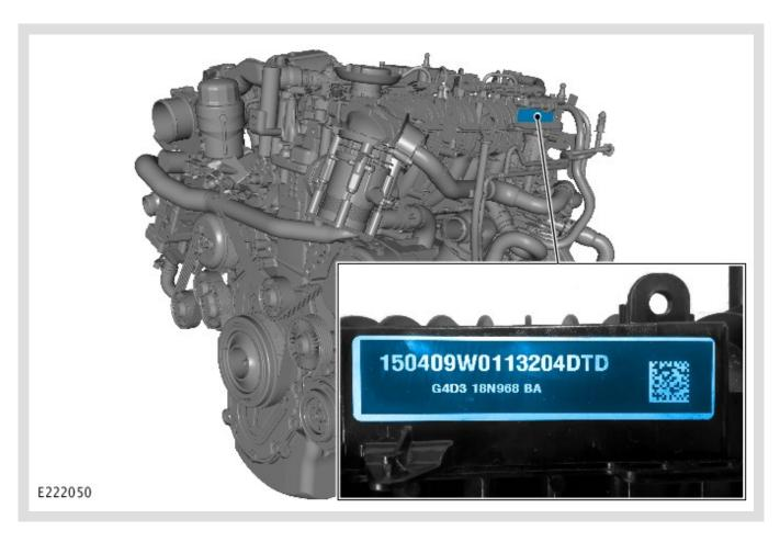
Locate and record the engine serial number.
