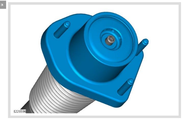
Install the new rear left shock absorber top mount.
