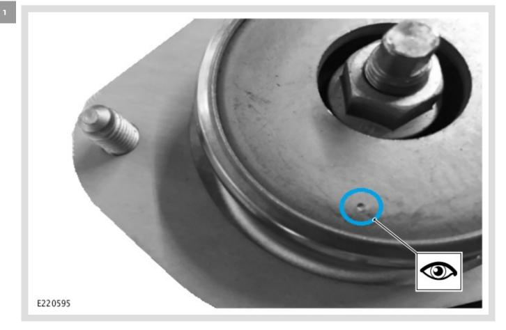
The new top mount should be identified with a 'dot' punch mark on the top plate.
