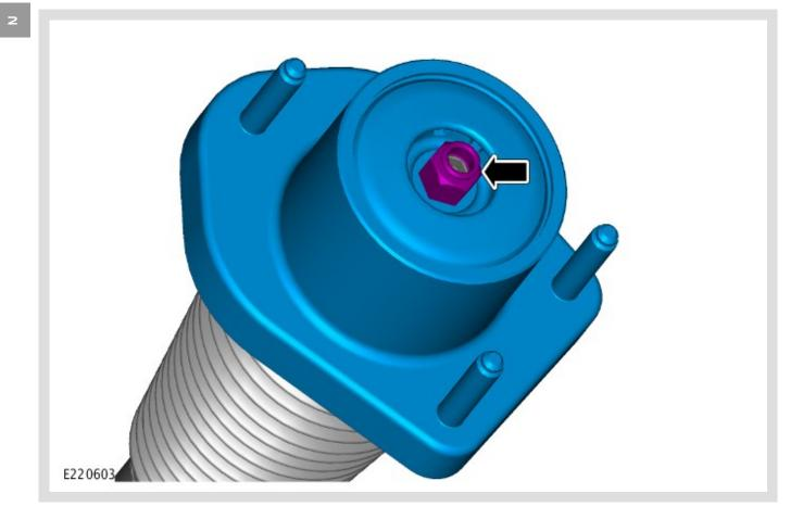
Remove the rear left shock absorber top mount.
