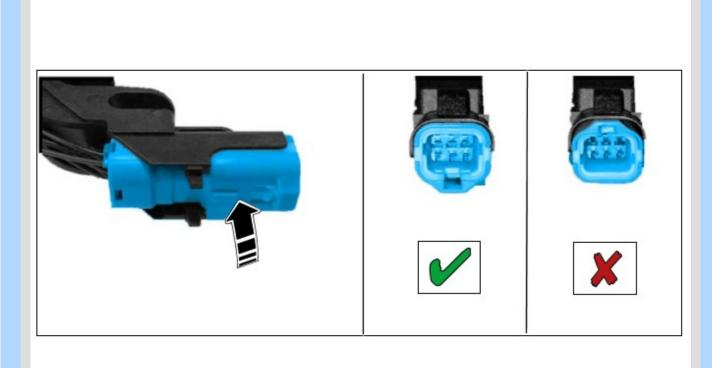
Clip the electrical connector into the handle strap inner ( $\checkmark$ ).
