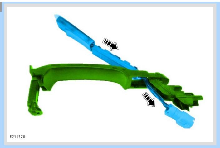
Insert the electrical connector through the door exterior handle strap inner.
