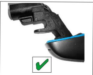
Make sure the rubber gasket sits flush against the handle base and the locating lug at the front of the gasket is installed into the hole in the handle ( $\checkmark$ ).
