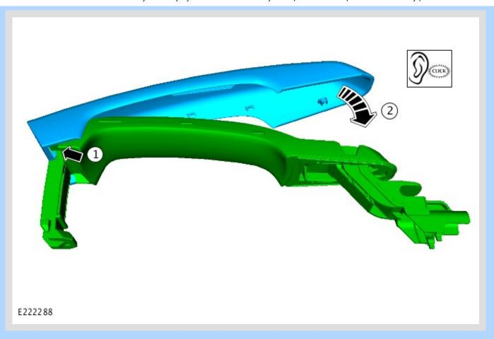
Assemble the inner and outer sections of the door exterior handle by clipping the 2 sections together.
