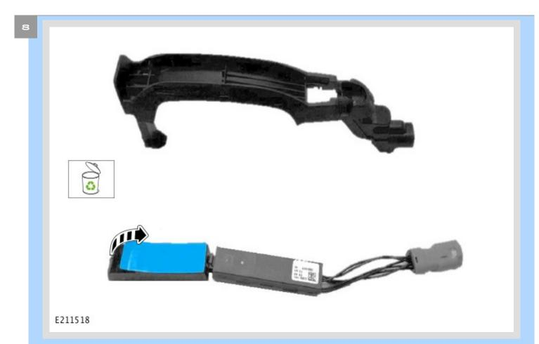
Prepare the door exterior handle strap inner and electronic module for assembly.
