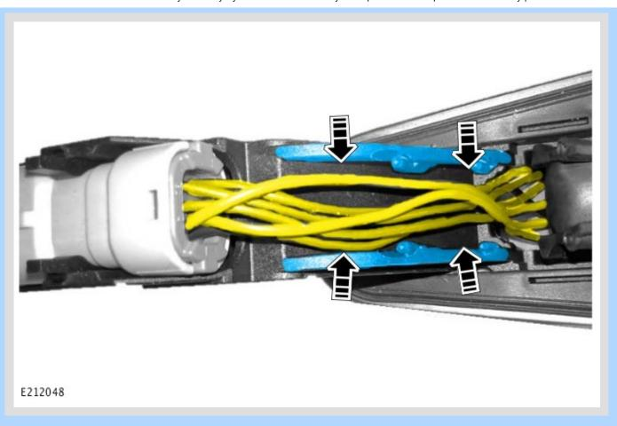
Make sure the wiring harness is positioned.
