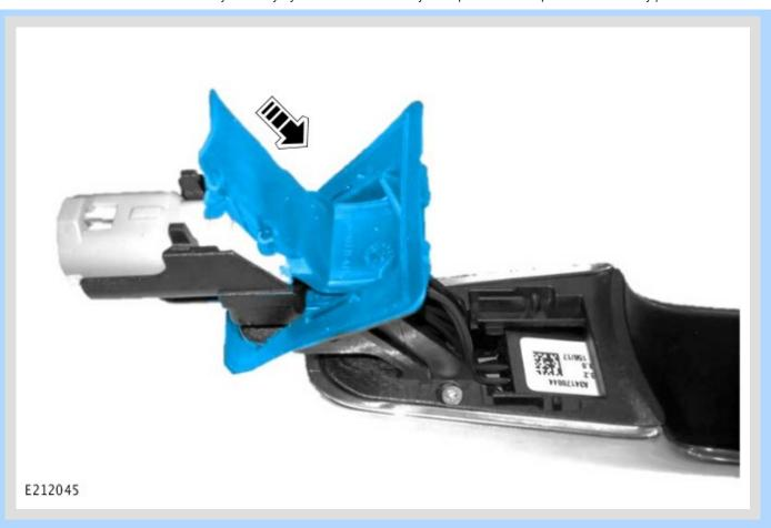
Start the installation of the door exterior handle gasket.
