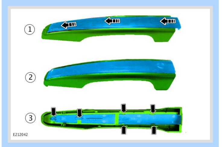
Install the painted door exterior handle insert into the door exterior handle cover (1).
