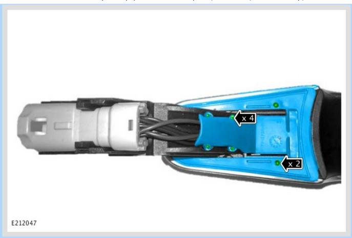
Install the rubber gasket onto the door exterior handle strap.
