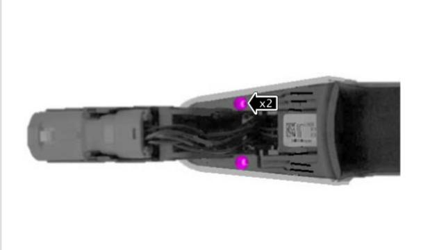
Install the 2 screws into the handle strap.
