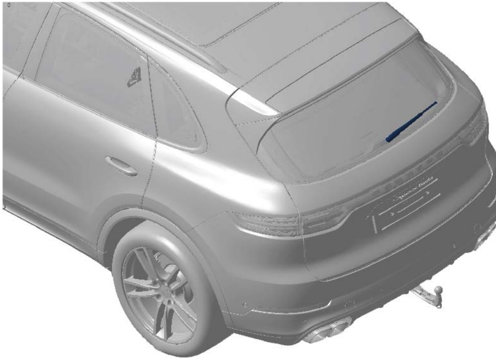
Installation position of wiper arm (shown on the Cayenne)
