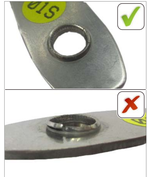
Checking cone for cracks
