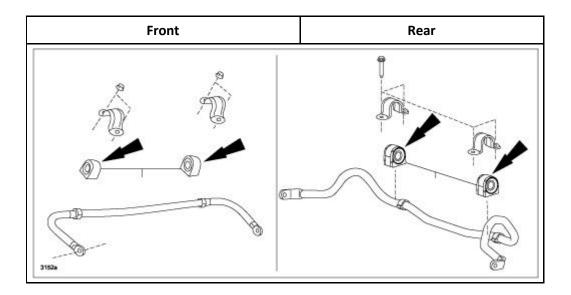
**NOTE:**To prevent noise from occurring, never apply any type of grease or lubrication to the front or rear stabilizer bushings.
