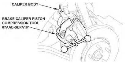
12. Press in the piston with the brake caliper piston compressor tool.
