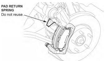
6. Remove the pad shims and the brake pads.
