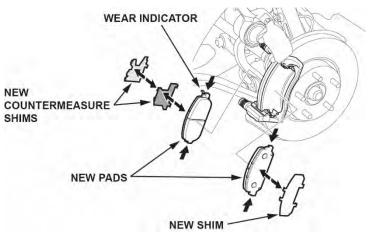
16. Install the new brake pads and pad shims, make sure the brake pad wear indicator is facing up.
