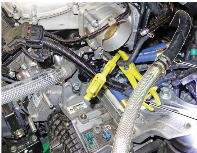
HEATER HOSE PUMP OUTLET HOSE
